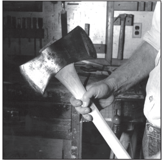
Figure 53—This handle is properly mounted on the shoulder. Compare this photo with the untrimmed handles in Figure 39 to see how low on the shoulder this ax head is mounted. There is no excess shoulder, and the handle is ready to be wedged.
