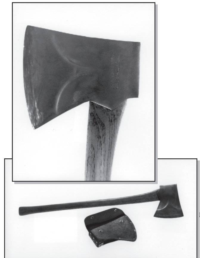
Figure 13—My favorite American felling ax, a True Temper Kelly Perfect with a Jersey head and 32-inch straight hickory handle.
