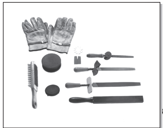
Figure 63 —Tools for sharpening (clockwise from top left) include leather gloves; ax-bit width gauges; 8-inch, 10-inch, and 12-inch mill bastard files; Carborundum scythe stone; Carborundum ax stone; file card; and grooved Carborundum sharpening stone. Natural Arkansas sharpening stones also work.
