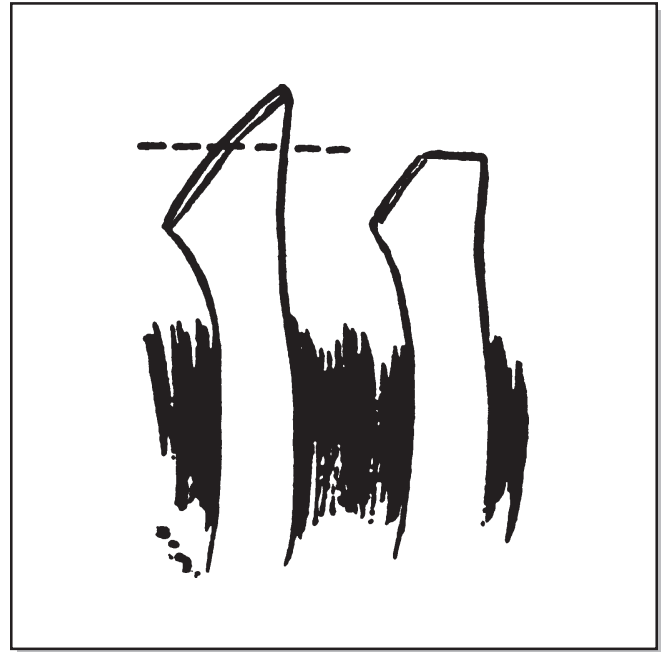
Figure 45—If you use a fawn's foot handle, saw off the handle about \frac{3}{4} inch from the butt end to provide a blunt surface for pounding with your mallet (drawing by Frederic H. Kock).
