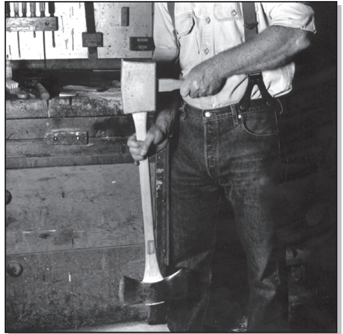
Figure 49—When the ax is properly hung, the bottom of the ax eye should rest on the shoulder of the handle. Drive the new handle into your ax head for a trial fit. Place the handle in the eye socket from the bottom. Use a large wooden mallet to strike the bottom of the handle squarely and firmly. This will draw the weight of the ax head up onto the handle. There's no need to rest the ax head or the handle against a solid base. Sight down the cutting edge to see if the ax edge is in exact line with the end of the handle (See Figure 31).
