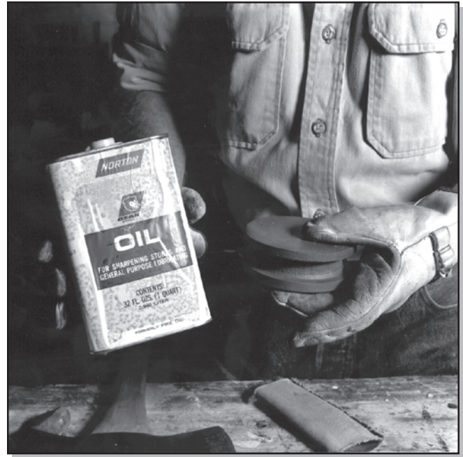
Figure 70—Use oil to float metal particles off ax stones made of Carborundum.
