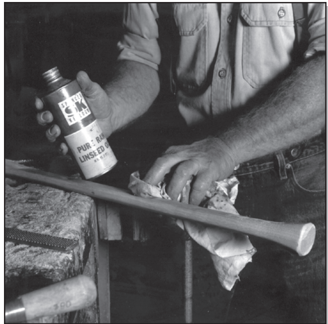
Figure 61—Apply a light coat of raw linseed oil if it is available, or boiled linseed oil if it is not. Tung oil will also work. A regular application of these oils will protect against drying and cracking. Wipe off the excess oil.
