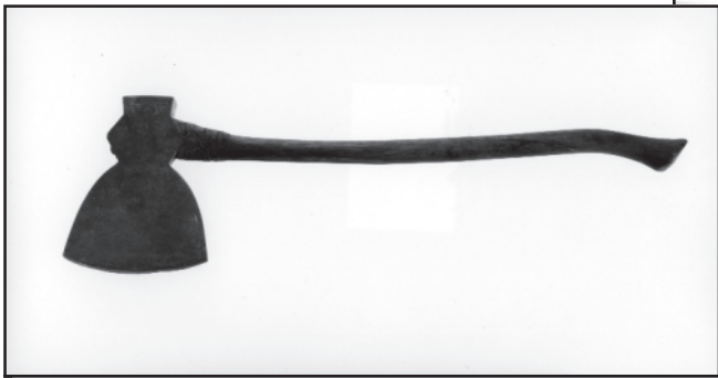
Figure 18e—A 19th-century shipwright's mast broad ax.
