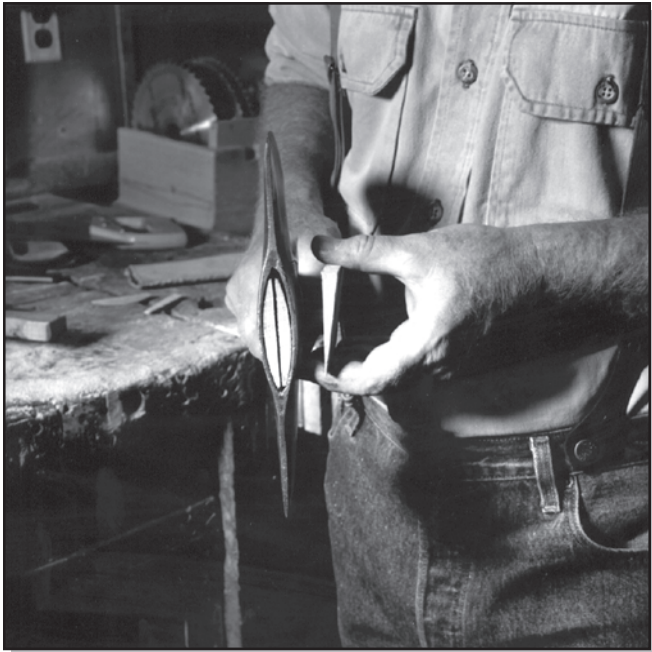
Figure 55—The fitted handle is ready for wedging. Use a correctly sized wooden wedge, usually made of well-seasoned yellow poplar or other hardwood. Avoid plastic or steel wedges.
