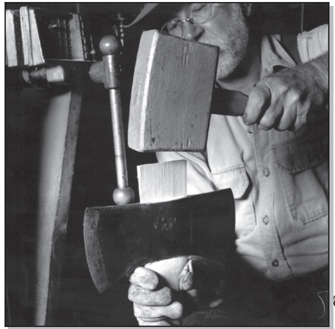
Figure 58—Insert the wooden wedge. Rest the handle bottom on something solid. Drive the wedge squarely and firmly into the kerf with a wooden carpenter's mallet. If you have set everything up properly, there should only be \frac{1}{4} to \frac{1}{2} inch of wedge protruding above the top of the handle when the wedge has been driven to the point of refusal. Use a coping saw to cut off any excess wedge.
