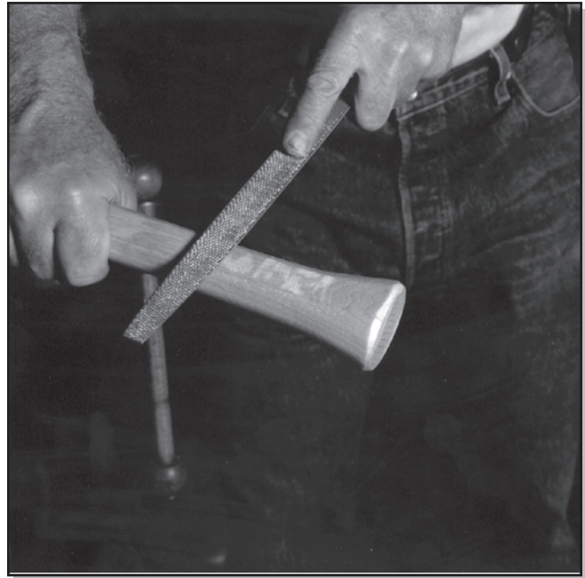
Figure 60—Rough up the lower 6 inches of the butt section of the handle with a wood rasp. This rough section will give purchase, or grip, to your stationary hand at the bottom of the ax handle.
