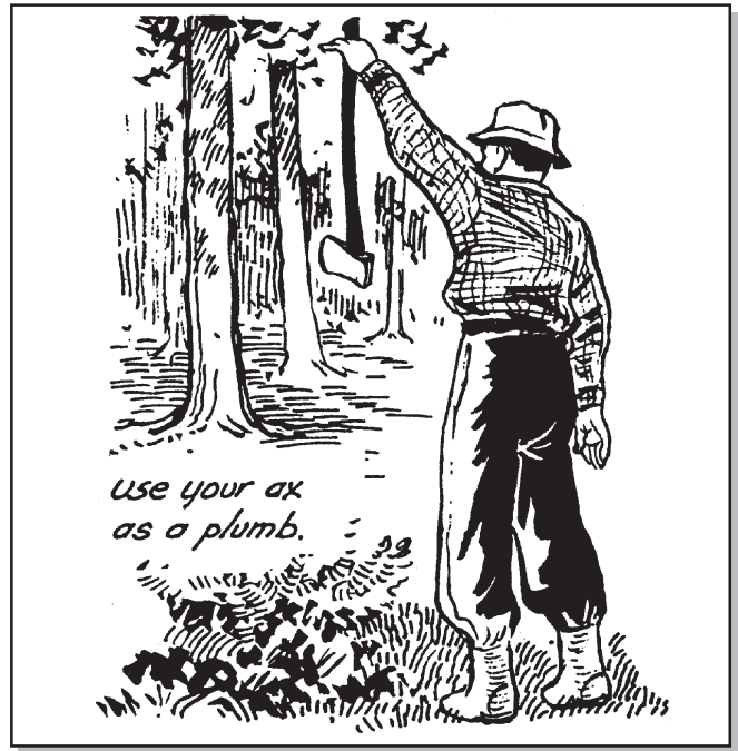
Figure 82—Using an ax as a plumb. A hard hat is also required here (drawing by Frederic H. Kock).
