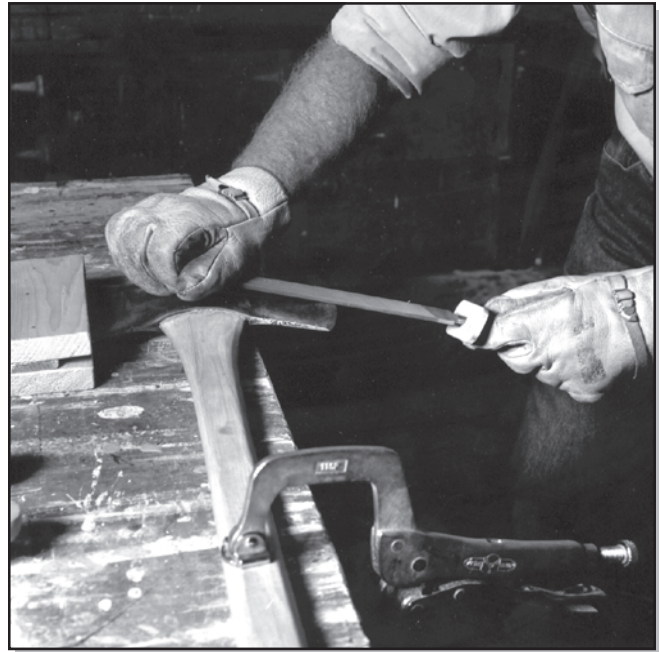
Figure 65—Clamp the ax to the bench at a comfortable height for sharpening.
