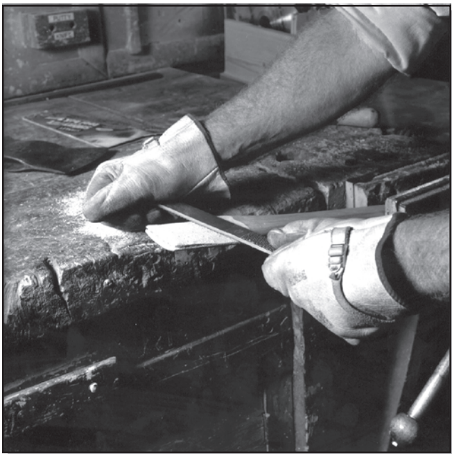
Figure 48—Using an aggressive wood rasp or a four-in-hand, start dressing down the handle to fit the ax-eye socket tightly. At this point, be careful not to split off the edges of the handle or to rasp off too much wood. Once it's rasped off, it can't be put back! It usually takes several repetitions of rasping and checking for fit to get everything just right.
