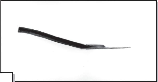
Figure 34b—A 19th-century S-bend broad ax handle.
