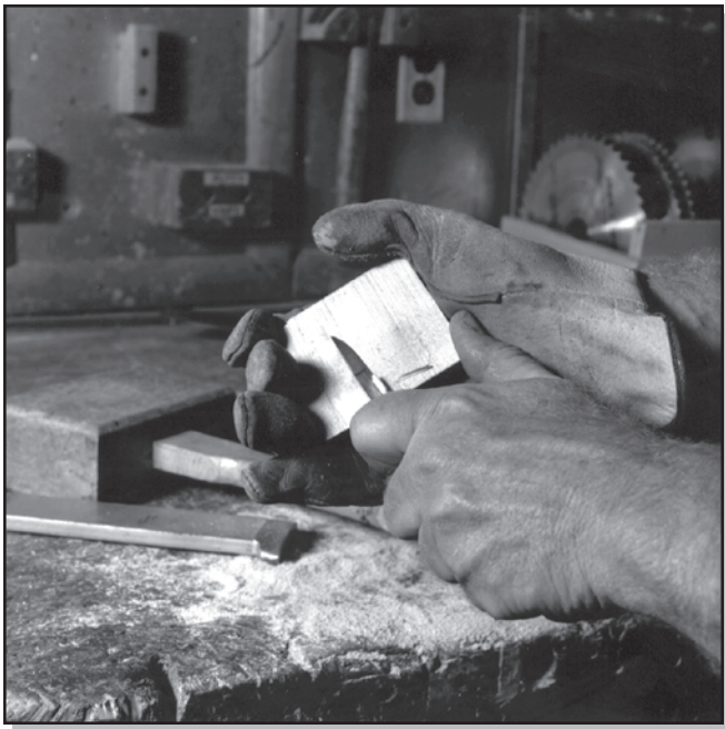
Figure 56—Sometimes the wedge is too thick for the saw kerf and ax eye. If so, thin the wedge out a little bit so that it can be driven almost full length.
