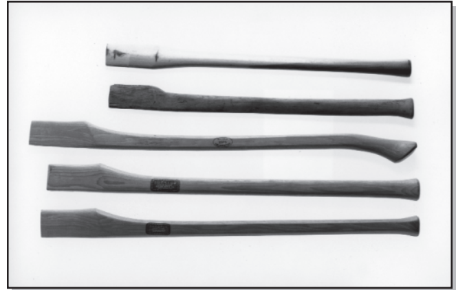
Figure 39—Some ax handles, from top: double-bit with too much heartwood; handmade 19th-century single-bit; the next three are new single-bit handles from O.P. Link—fawn's foot octagonal, straight oval, and my favorite, straight octagonal slim-taper.
