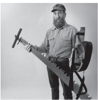
Figure 7—The sawguard is rolled and ready to be applied to the saw.
