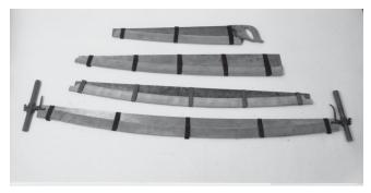
Figure 2—Crosscut saw guards properly applied using 1-1/2-inch fire hose. Velcro-style fasteners secure the straps.
