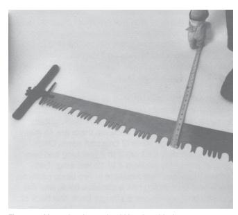
Figure 5—Measuring the saw's width at its midpoint.
