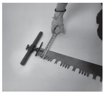
Figure 4—Measuring the width of the saw from the cutters to the back.
