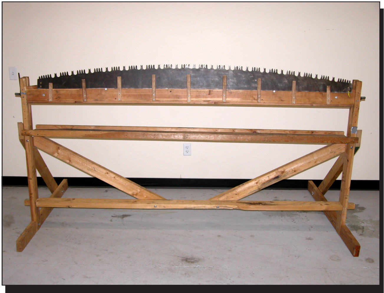
Figure 7—Freestanding crosscut saw vise.
