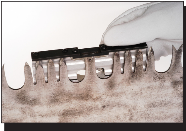
Figure 2—A saw raker fits into the slot of the adjustable raker gauge for filing.
