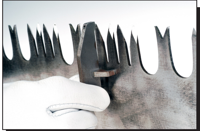
Figure 6—The adjustable spider gauge is used to determine the amount of set in a tooth. This spider gauge can be adjusted by using an allen wrench to turn the top screw to the desired tooth set.
