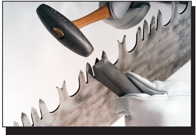
Figure 5—Hand-held anvils are less cumbersome than the tooth-set tool. They may be preferred by experienced saw filers.
