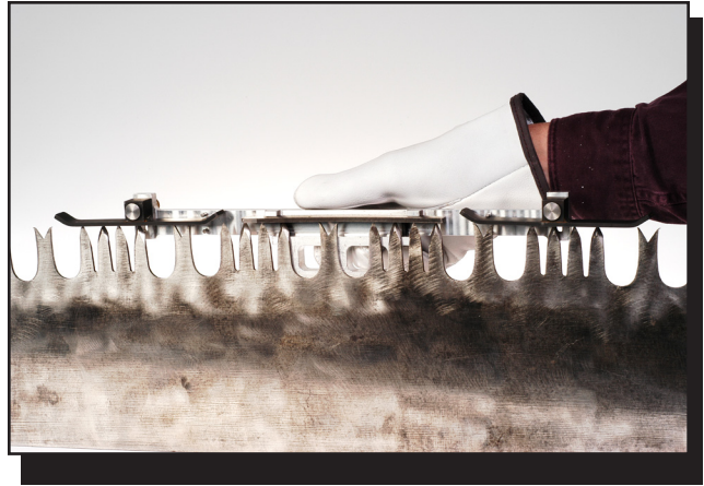
Figure 1—The jointer allows a saw's teeth to be filed to a uniform height before the cutting teeth are pointed (sharpened). Long jointers, such as the one shown here, help maintain the arc of the saw better than short jointers.
